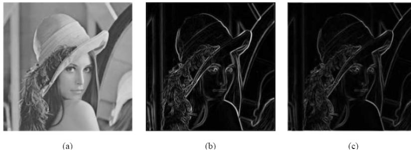
Figure 8. Gradient-based edge maps of Lena image. (a) Original image, (b) the gradient edge map implemented on square architecture, and (c) gradient map implemented on SA
